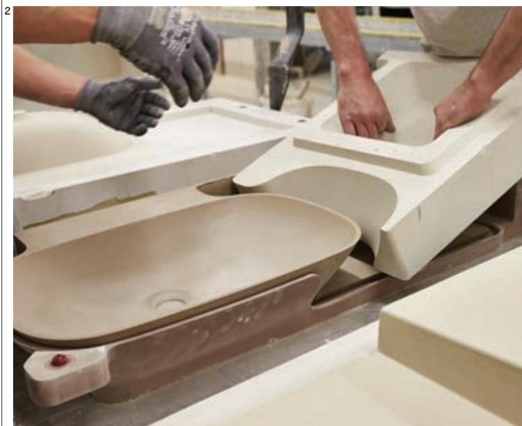
**1. Laufen craftsman hand finishing the new range of bathroom fittings designed by Konstantin Grcic and made from SaphirKeramik, the revolutionary new ceramic material which allows elements to be ultra thin**
